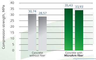
After 45 freezing and thawing cycles, concrete of B25 class reinforced with **MicroArm 12** mm fiber showed strength of 33.93 MPa. The strength loss was **4.23%** which is less than the **5%** value stipulated by ДСТУ Б В. 2.7-49-96 standard.
