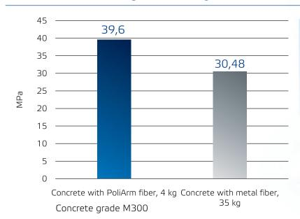
The specimen of concrete prepared with **4 kg PoliArm polypropylene fiber** shows much higher bending tensile strength than the identical specimen of concrete prepared with 35 kg metal fiber (calculated as per 1 m<sup>3</sup>).
