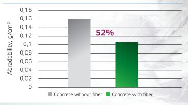
Abradability of M250 concrete with **MicroArm 12** mm fiber added at the rate of 0.9 kg/m<sup>3</sup> reduced by **52%** as compared with abradability properties of concrete without fiber.
