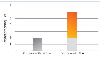
M250 concrete with **MicroArm 12** mm fiber added at the rate of 0.9 kg/m3 showed improvement of concrete waterproofing properties to **W4-W6** grade as compared with M250 concrete without fiber having waterproofing properties of **W2** grade.
