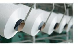
**TM Fiber polypropylene yarn** is high-strength multifilament yarn having a linear density **of 900 to 3600 denier.**
