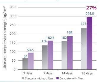
Specimens of M200 concrete with **MicroArm 12** mm fiber on 28<sup>th</sup> day showed compression strength gain of **27%** as compared with the concrete of the same grade without fiber.
