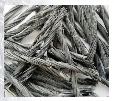
X Mesh™ Fiber – structured synthetic macrofiber made of oriented polypropylene copolymer in the form of twisted hard fibers, treated with a special compound that improves adhesion to concrete grout.
