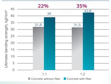
All specimens of M200 concrete with addition of **MicroArm 12** mm fiber at the rate of 0.9 kg/m<sup>3</sup> showed bending tensile strength gain of **22%** to **35%** without increase of cement dosage.
